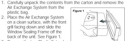
back of the unit. See Figure 1. 3. Remove the two Plastic Extender Panels from the plastic bags and
